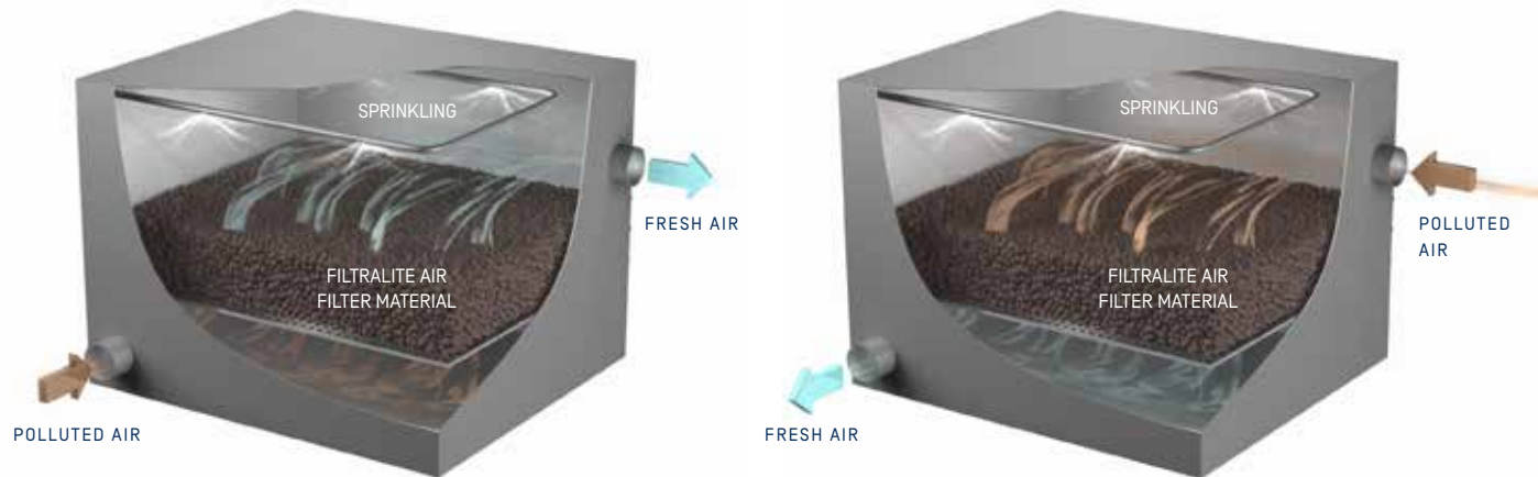
Upstream system. Polluted air is pushed upwards through the filter while sprinkling water drip downwards.
