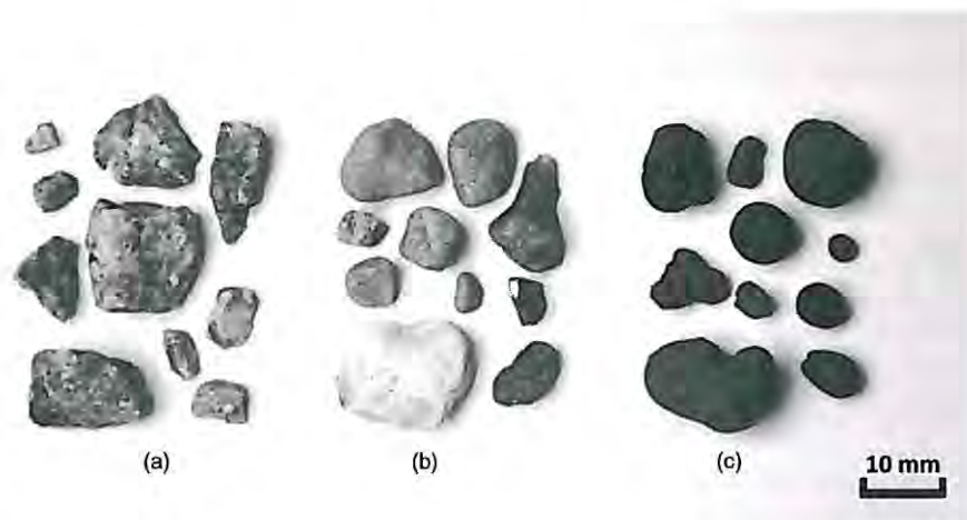
Fig. 1. Porous materials used in the tracer experiments: (a) granite; (b) gravel; (c) Leca
